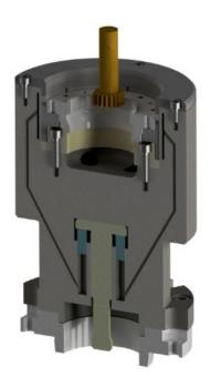
area is very short. We designed a hydraulic chuck in combination with a changeable back stop and slotted collet. This gives the customer options to clamp different diameters and components with one hydraulic chuck. This hydraulic chuck is used to machine the spline in the "Gear Shaping" process on a Liebherr machine.
