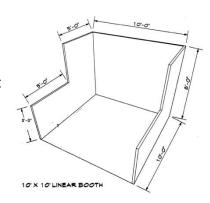
(3.05m) has become the de facto standard in the United States. Therefore, unless constricted by space or other limitations, Linear Booths are most commonly 10ft (3.05m) wide and 10ft (3.05m) deep, i.e. 10ft by 10ft (3.05m by 3.05m). A maximum back wall height limitation of 8ft (2.44m) is specified to prevent display materials from imposing on neighboring exhibits behind the back wall.
